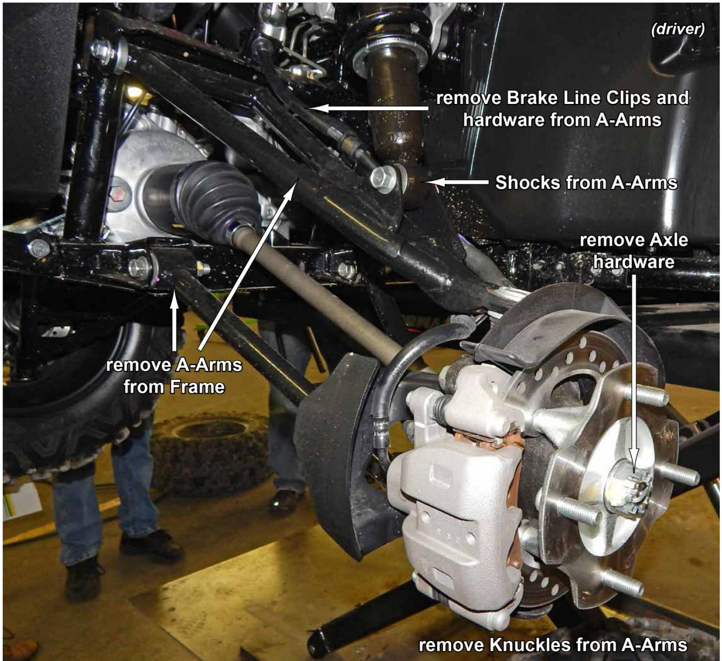
**Step 1.** Securely jack up your machine and remove the front wheels.
