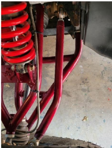
Next, make sure the jam nut is not installed on the inner tie rod (or heim joint), and push your stock tie rod boot on to the 14 mm shaft of the inner tie rod end, then screw on the jam nut. Make sure the
