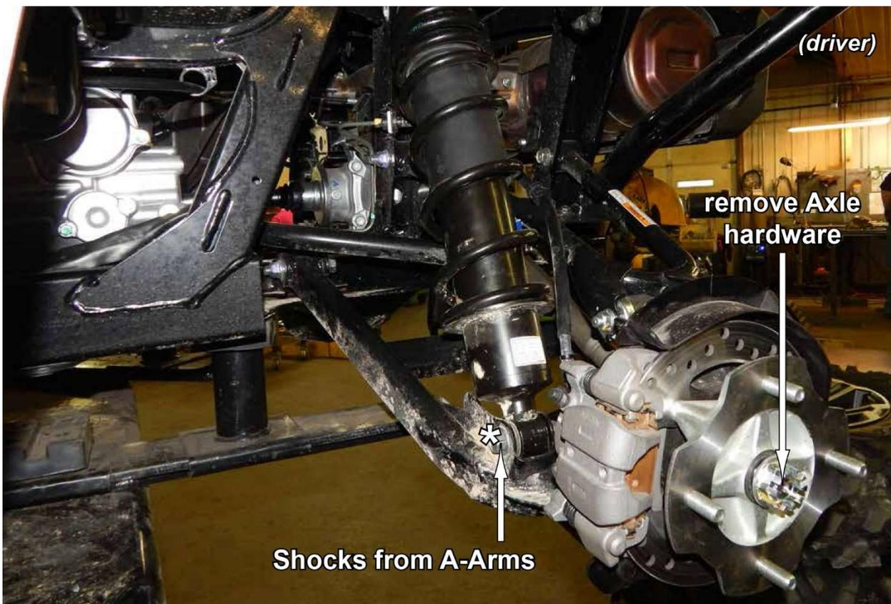
**Step 1.** Securely jack up your machine and remove the rear wheels.
