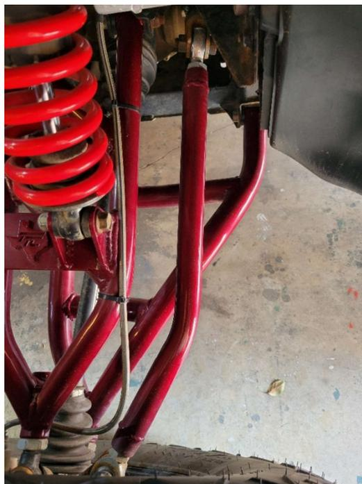
Next, make sure the jam nut is not installed on the inner tie rod (or heim joint), and push your stock tie rod boot on to the 14 mm shaft of the inner tie rod end, then screw on the jam nut. Make sure the boot is properly installed and seated in the groove on the rack and pinion, then secure it tightly with a zip tie.
